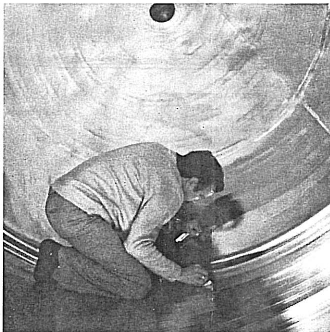
Figure 5. Electropolished interior surface of a tank. Notice the reflection attained by the process.
